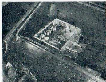
The electronic calculating unit installed in the boot of the TR.2.
