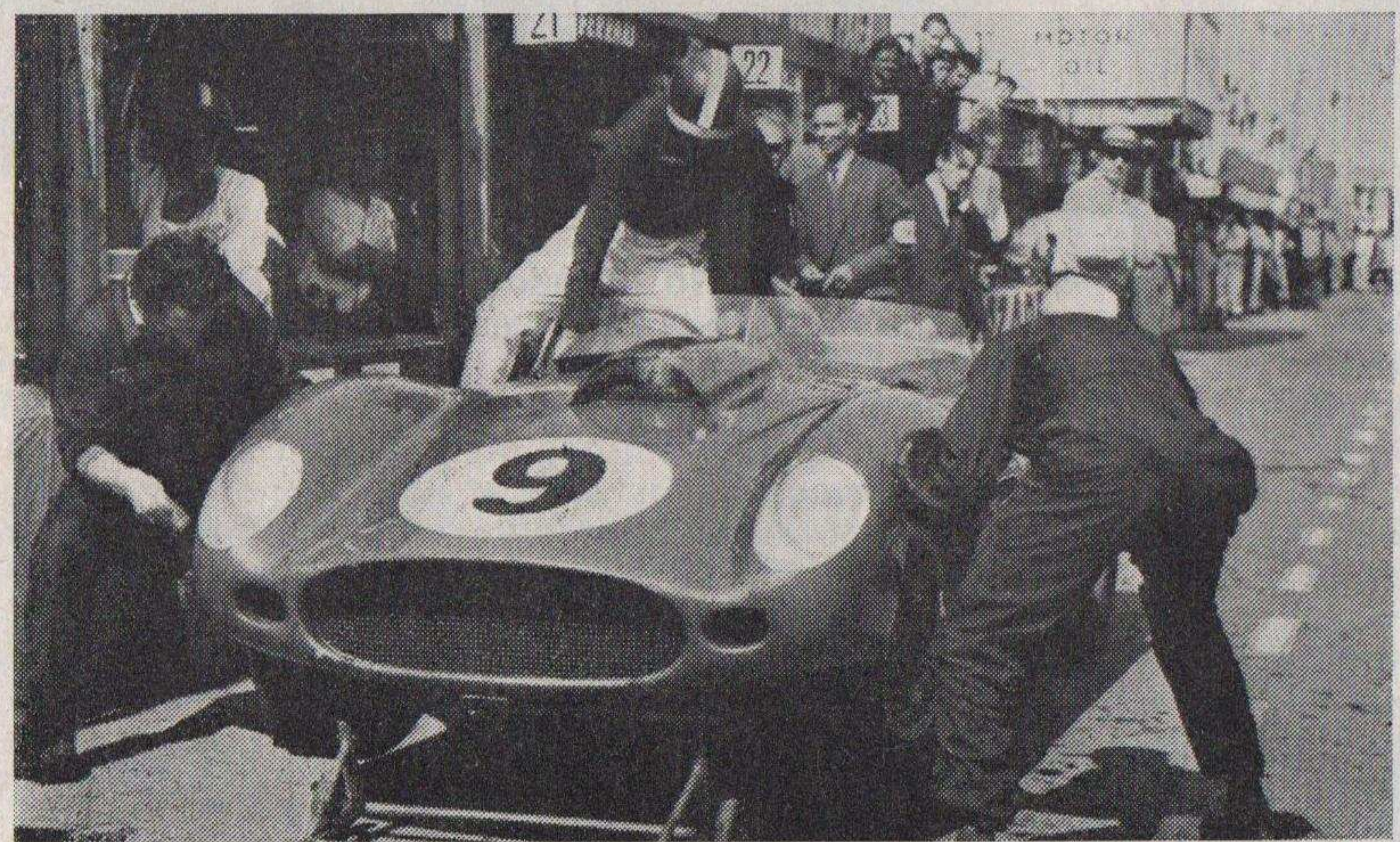
The drama of a pit stop with Tony Brooks leaping into the cockpit of the Testa Rossa Ferrari as mechanics give a final whack to the knock-on wheels. This was during the 1959 race, and the blood-red Italian sports car had been re-fuelled, had all four wheels changed and the nearside front brake adjusted in 95 seconds. Brooks later took over the second Ferrari team car with Olivier Gendebien and finished third behind the Moss-Shelby-Fairman Aston Martin and the Porsche driven by Wolfgang von Trips.
