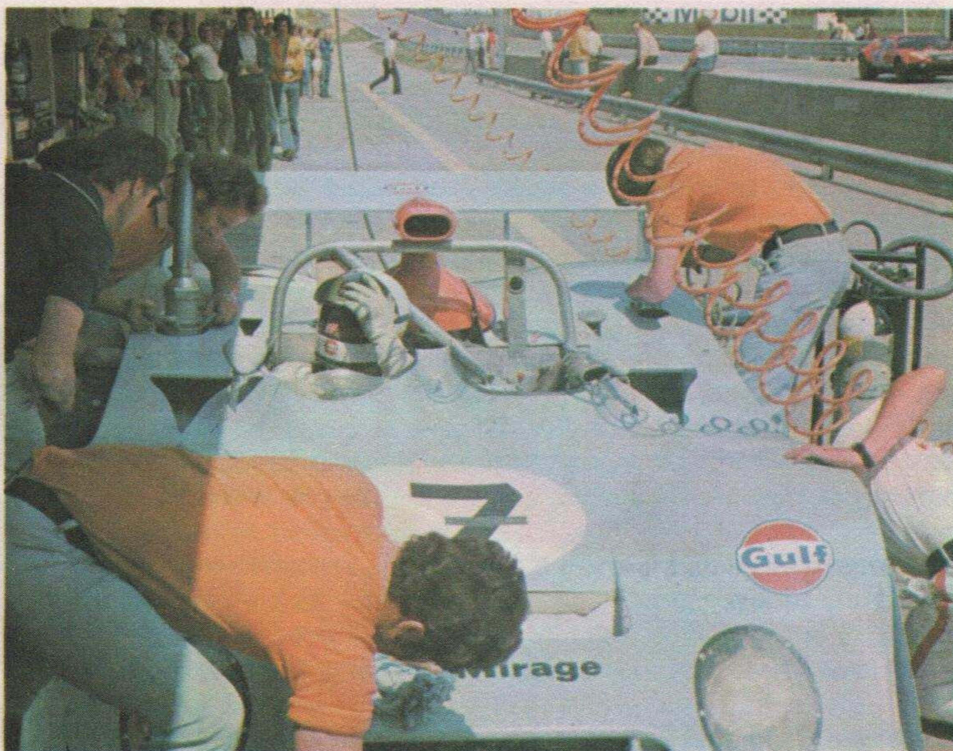
Mechanics jump into action as Derek Bell brings the Gulf-Mirage to a halt during the Austrian 1,000 kms race in June. One attaches the petrol filler hose while others concentrate on their own jobs. The coiled wires are attached to power tools used to remove wheel nuts.
