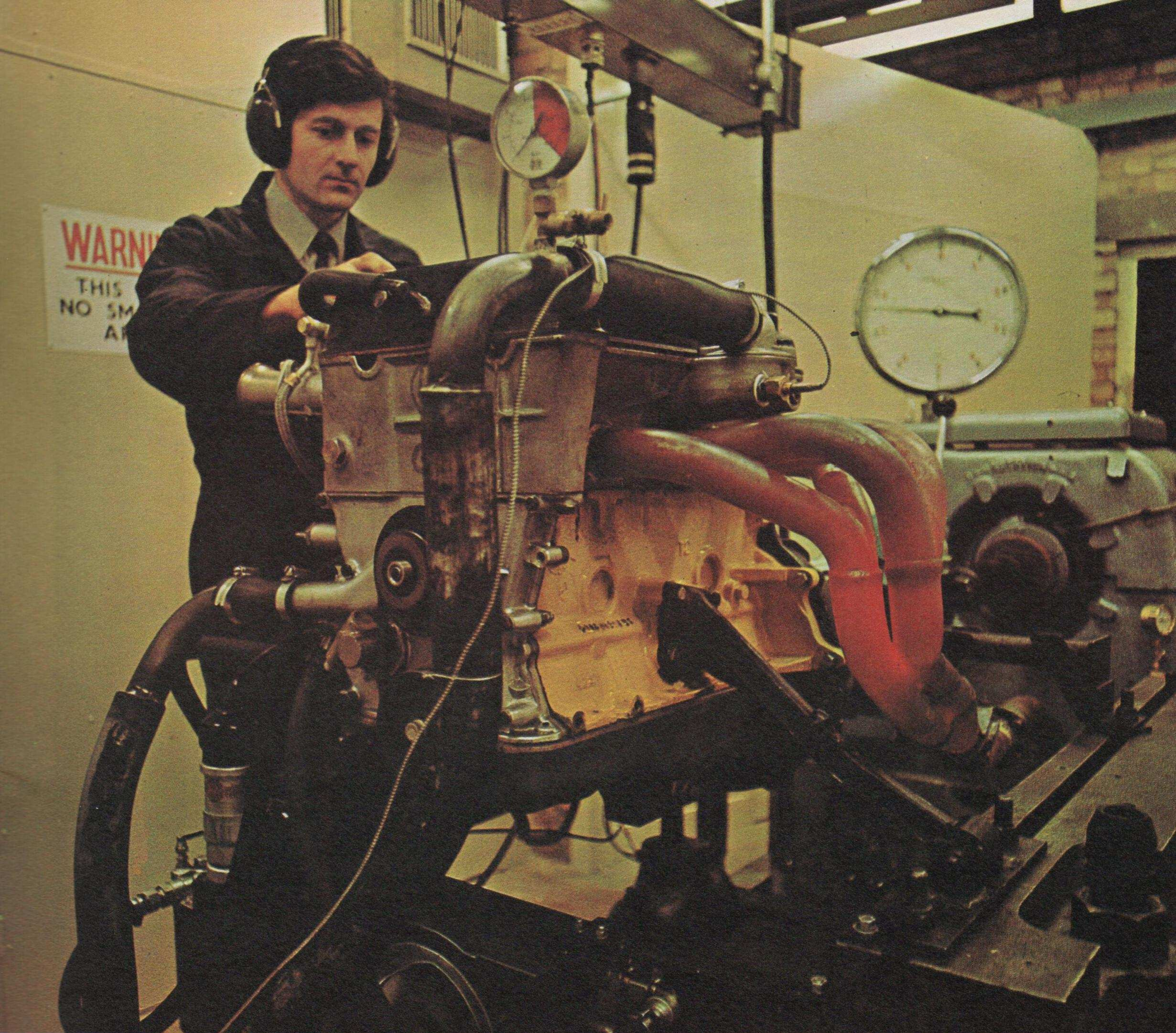
Ford bench-test a Lotus twin-cam engine on Castrol.
