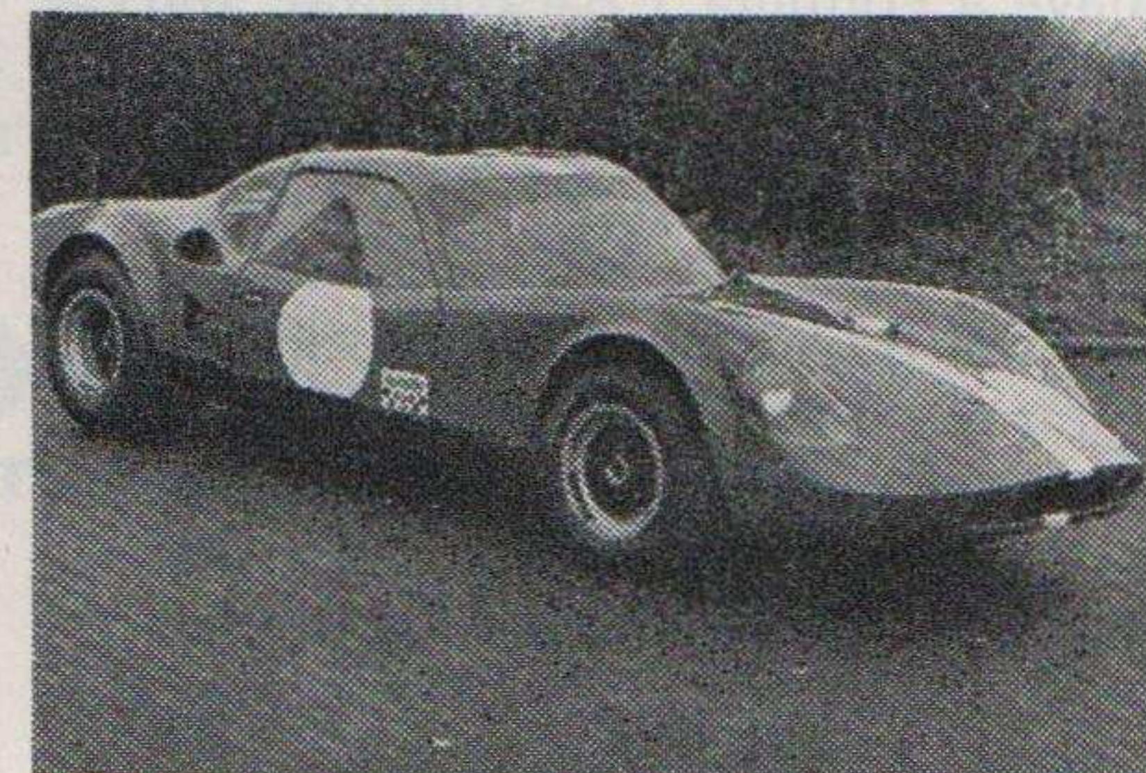
British 2 litre challenger in the Group 4 category. The highly successful Chevron B8 uses a BMW engine.
