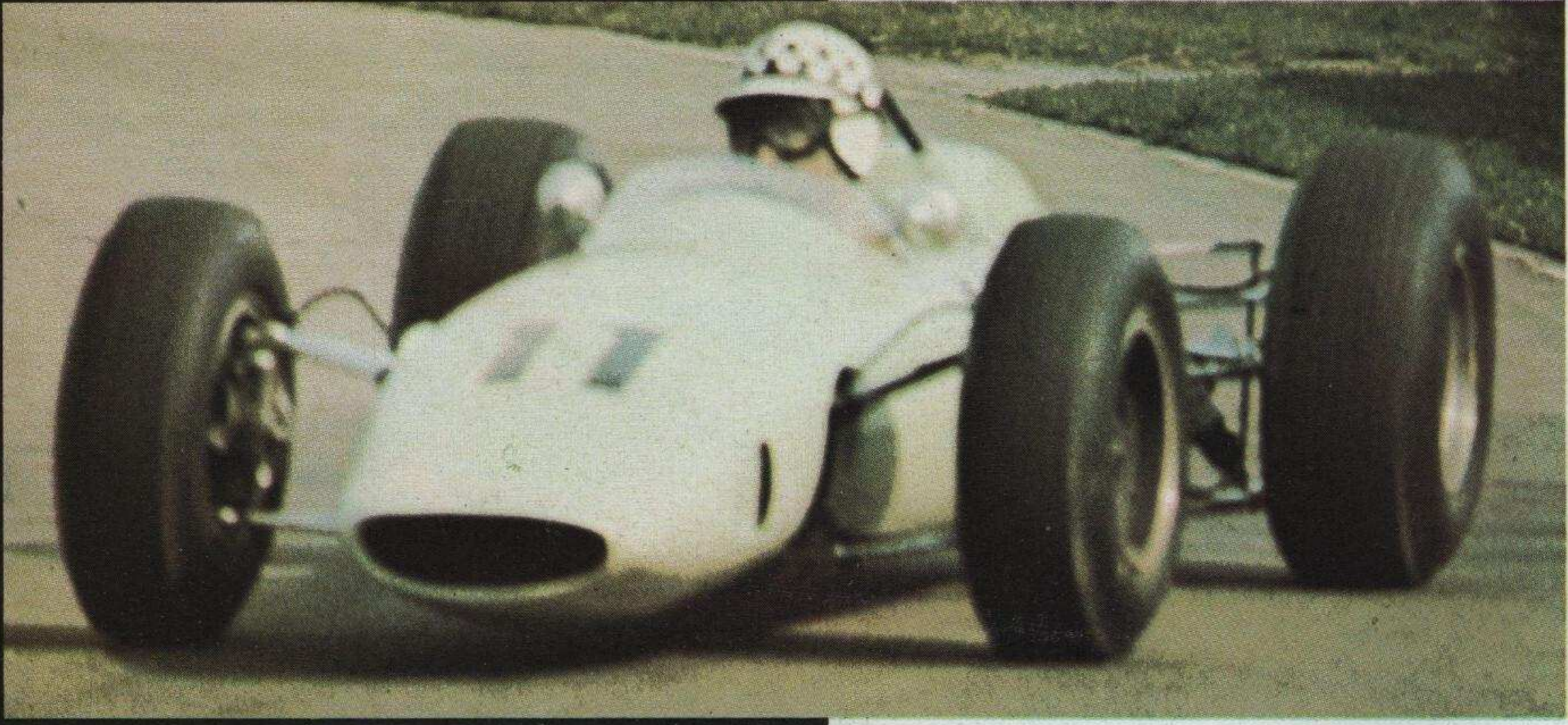
The BRP, a monocoque racing car designed and constructed by the London-based British Racing Partnership to replace the team's 'production type' Lotus 24s
