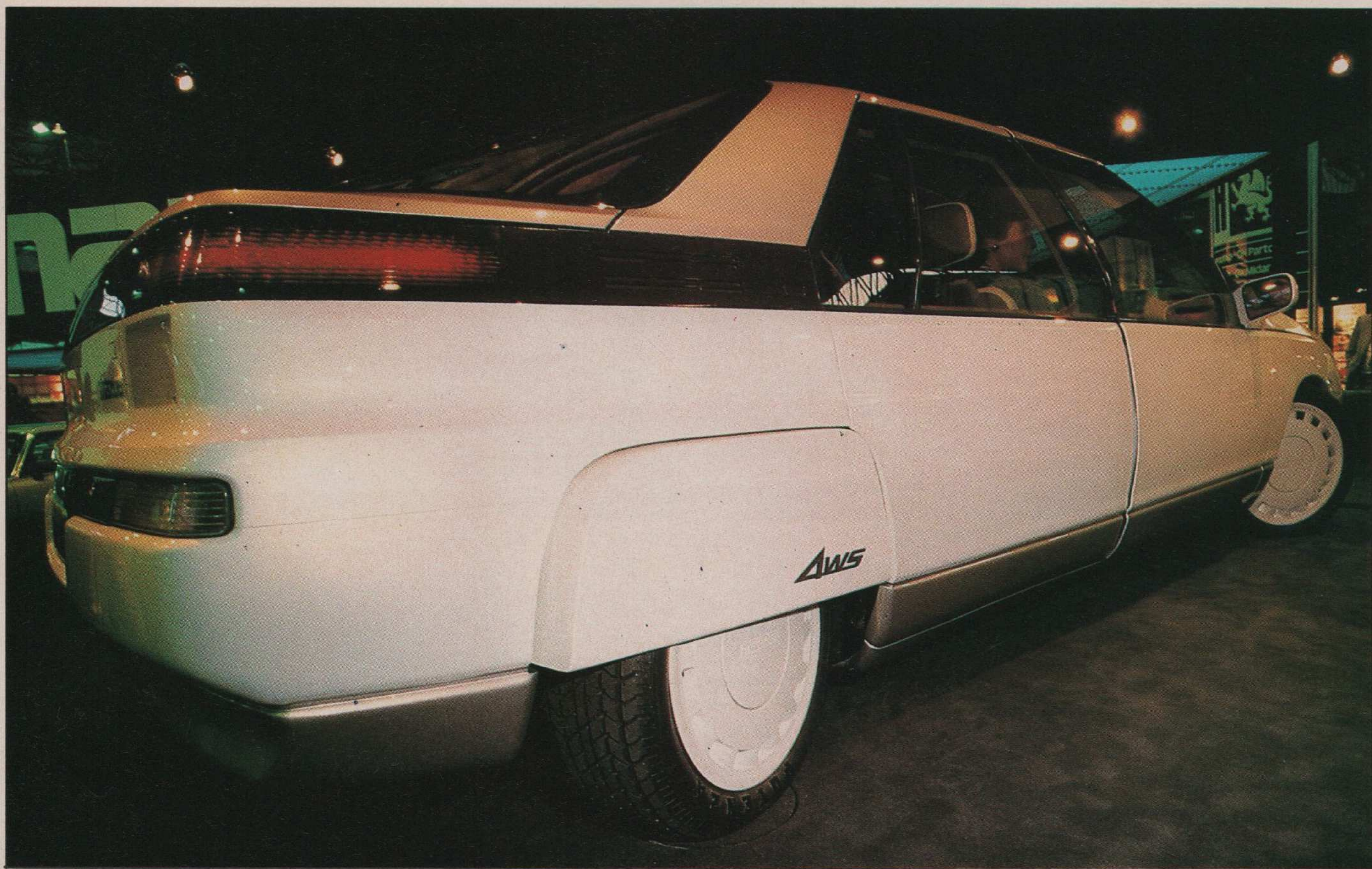
Mazda MX-02 experimental car is fitted with four-wheel steering. The Japanese claim that the effect is to enhance a car's stability
