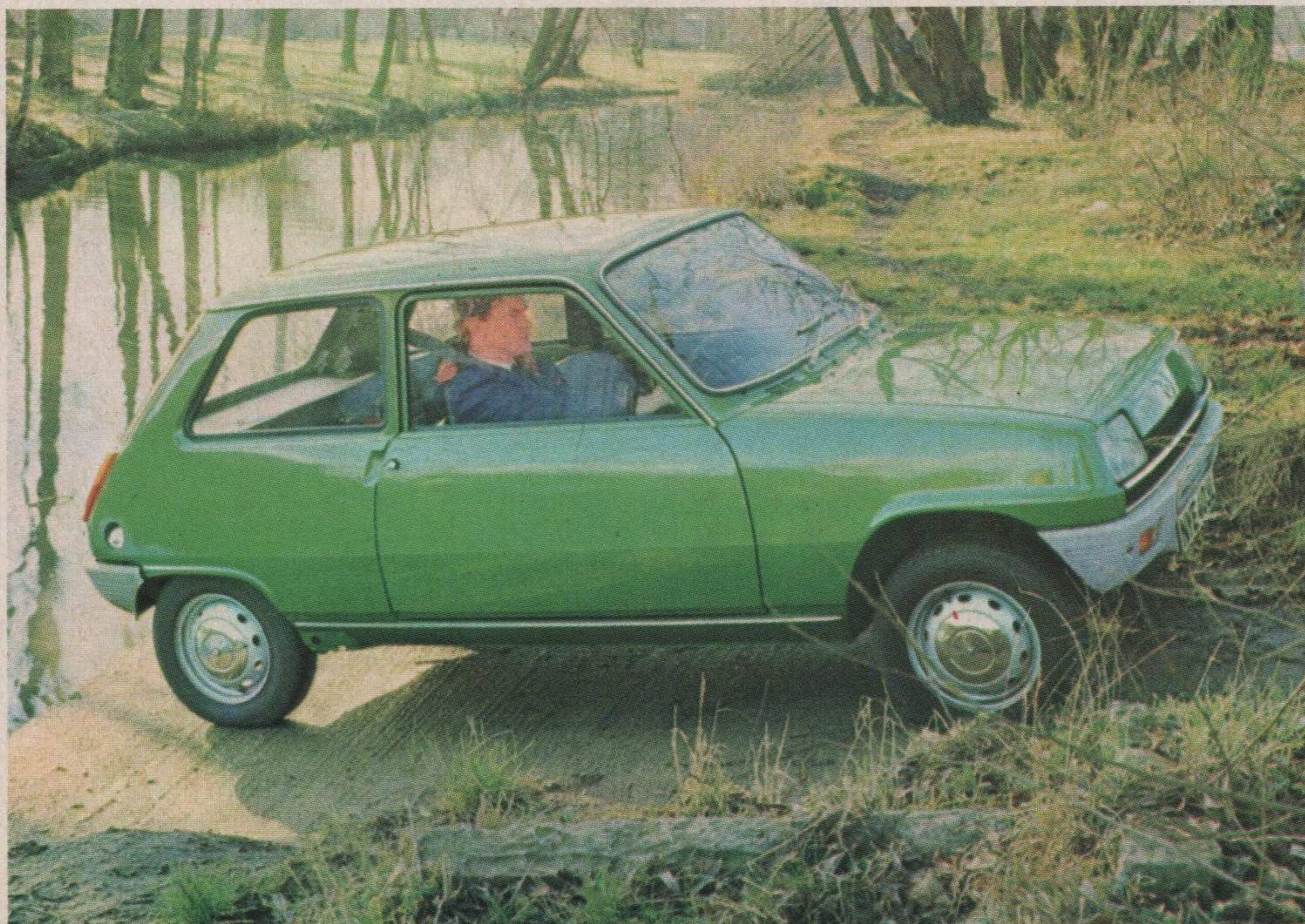
Below: A 1970s approach to small car design has produced the Renault 5TL with 956 c.c. engine driving the front wheels, a lift-up rear door and a fold-down rear seat
