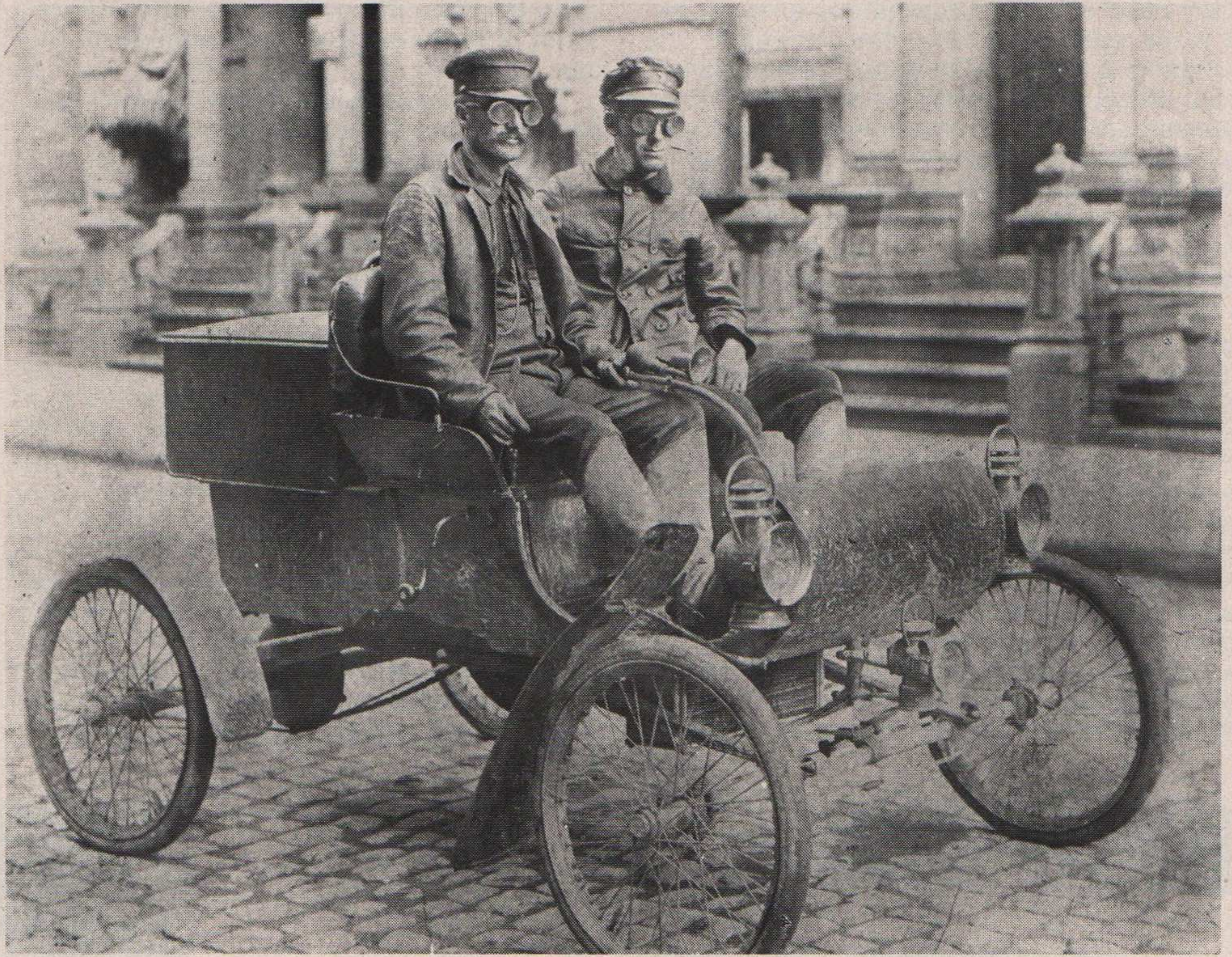
Above: This 1903 curved dash Oldsmobile, with its single-cylinder, under-floor engine, was typical of the American "gas buggy". Right: Rudge detachable centre-lock wire wheel of 1907, with a puncture preventer to knock nails and flints off the tyre
