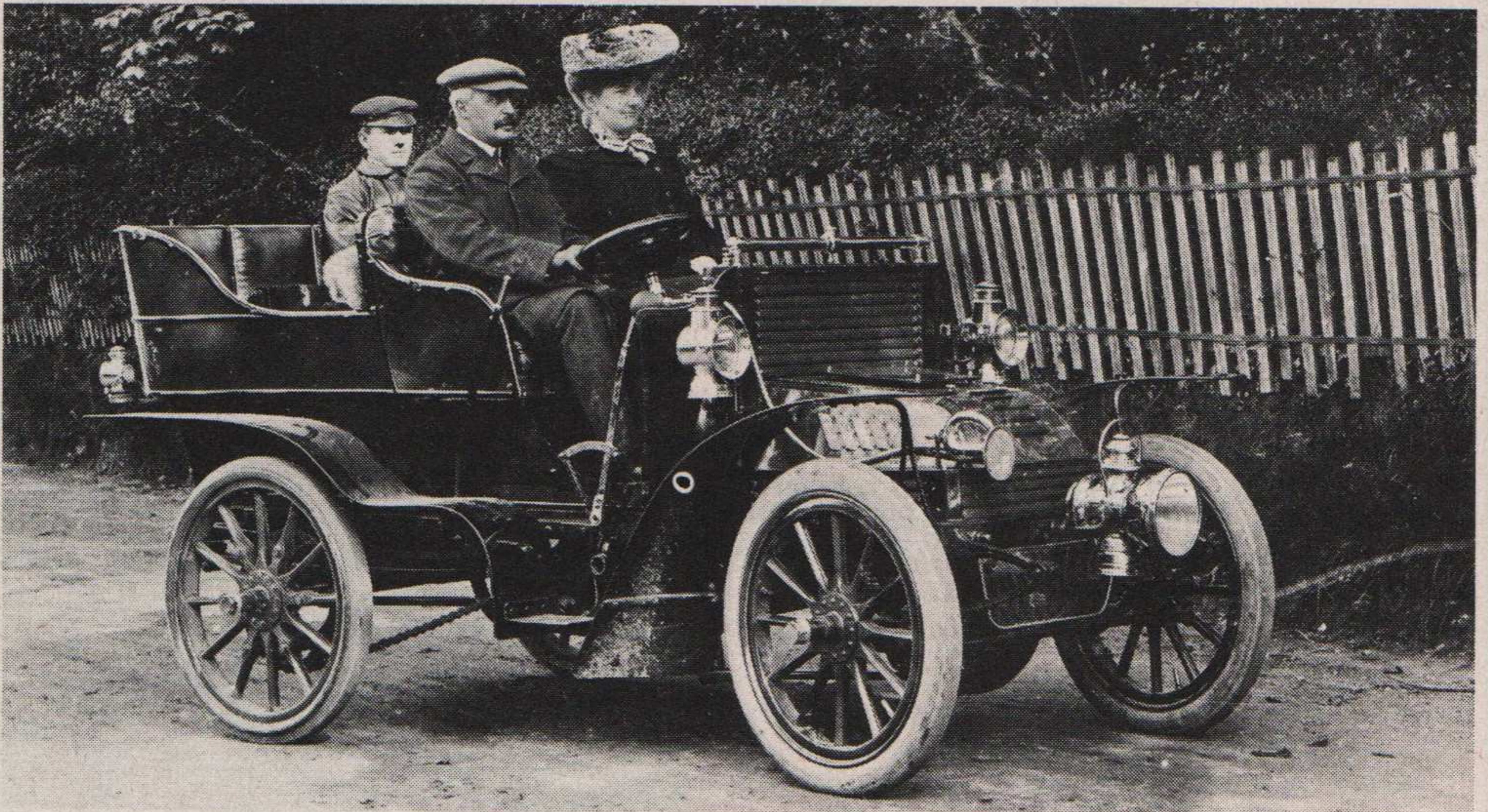
Above: The 1903 Brooke 14 h.p. had a "pudding basin" steering wheel, and a patent Estcourt dashboard-mounted radiator
