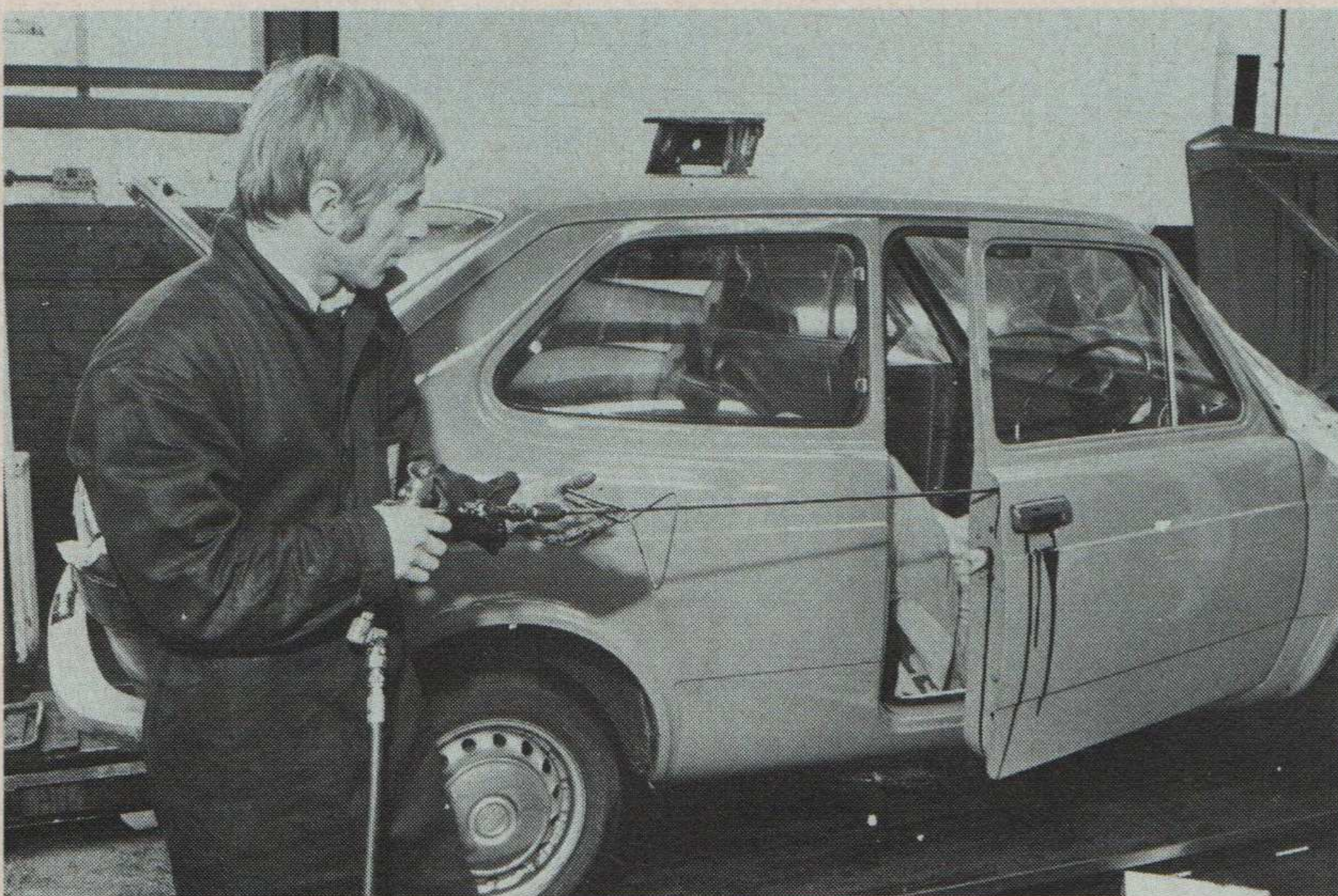
One of the biggest problems of the mass produced cars of the post-War period has been rust, and current cars are still plagued by it. Though not completely solving the problem, processes like Ziebart which treat internal and underbody surfaces prone to rusting, bring the rust-free car a step nearer
